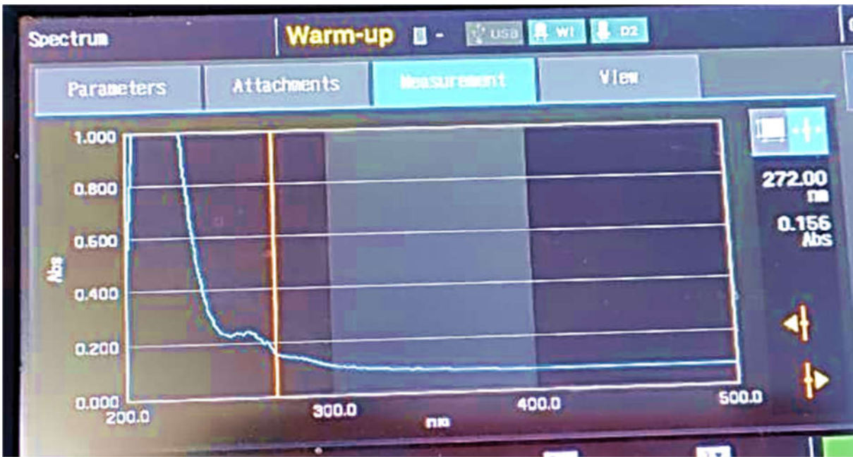
Fig.2: spectrum of Miconazole Nitrate in Ethanol
