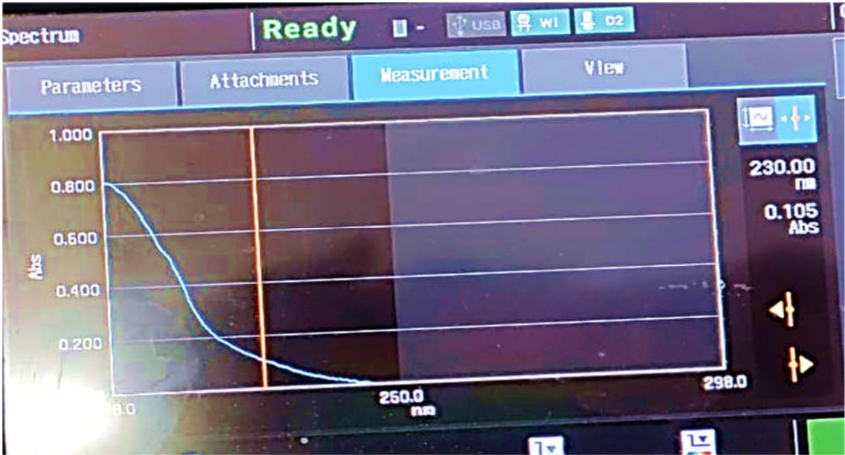
Fig. 3: Spectrum of Miconazole Nitrate in Phosphate Buffer pH 7.4
