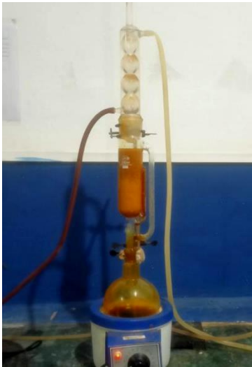
Figure 5 :Soxletation of Curcuma Longa with Hydro alcoholic solvent
