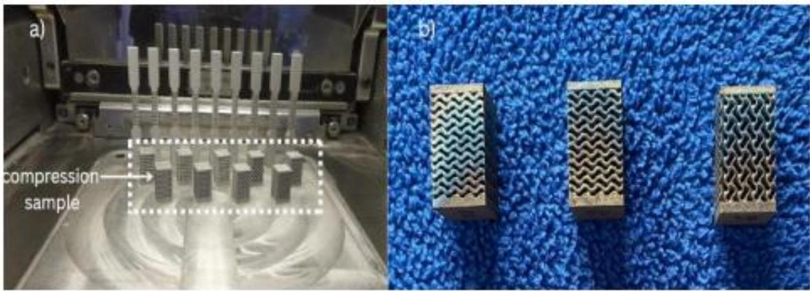
Figure 4.4 a), Figure 4.4 b) Gyroid Specimen fabricated using Ti6Al4V from Amison Engineering, Pune
