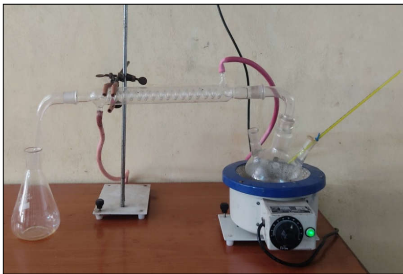
Fig.2. Experimental Setup of MDPB Pyrolysis Process
