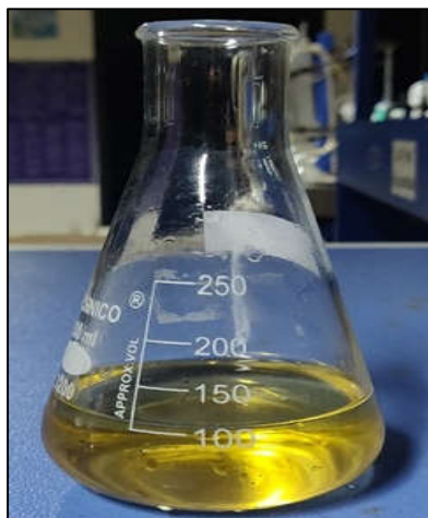
Fig.7.Liquid fuel obtained from PP Pyrolysis
